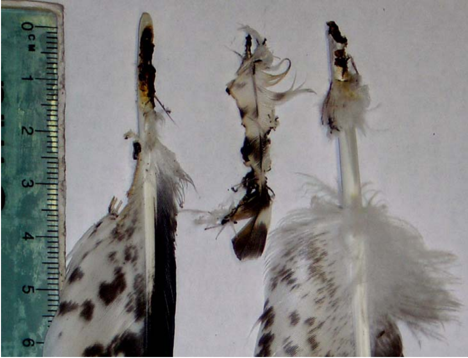
Figure A7) Typical charring of feather calamus (from an electrocuted Harris' hawk in this case).
